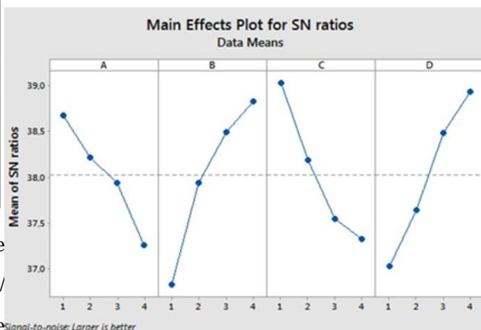
Fig. 2. Variation of S/N ratio for each parameter
